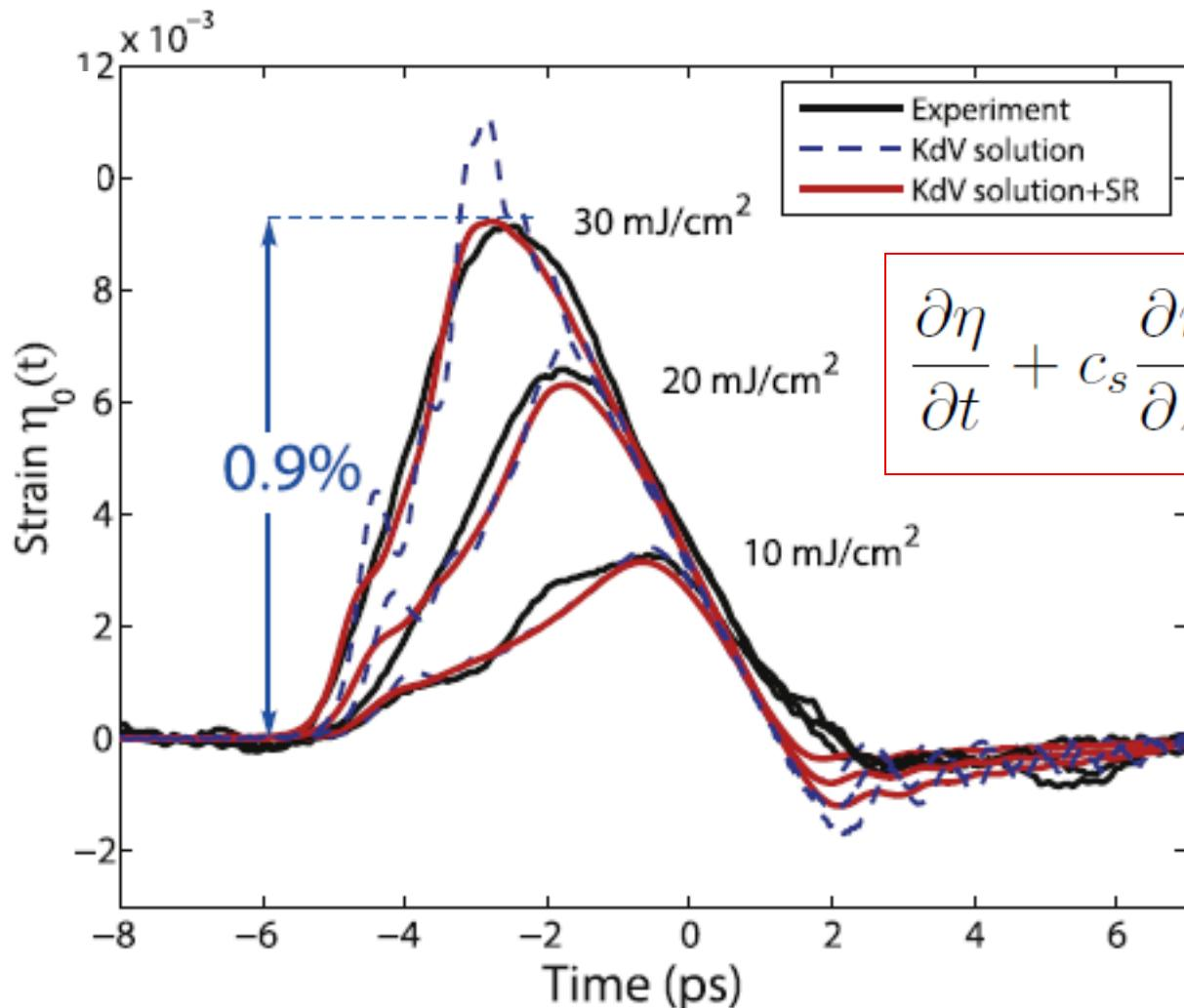
$$\frac{\partial \eta}{\partial t} + c_s \frac{\partial \eta}{\partial z} + \gamma \frac{\partial^3 \eta}{\partial z^3} + \frac{C_3}{2\rho c_s} \eta \frac{\partial \eta}{\partial z} = 0$$
