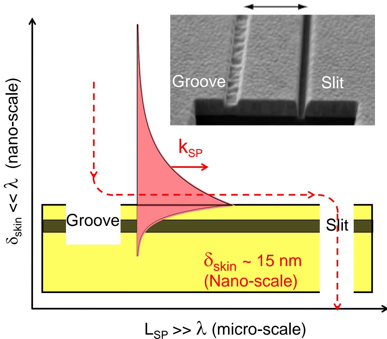
Sub-wavelength slit-groove pairs produced by the focused ion beam
