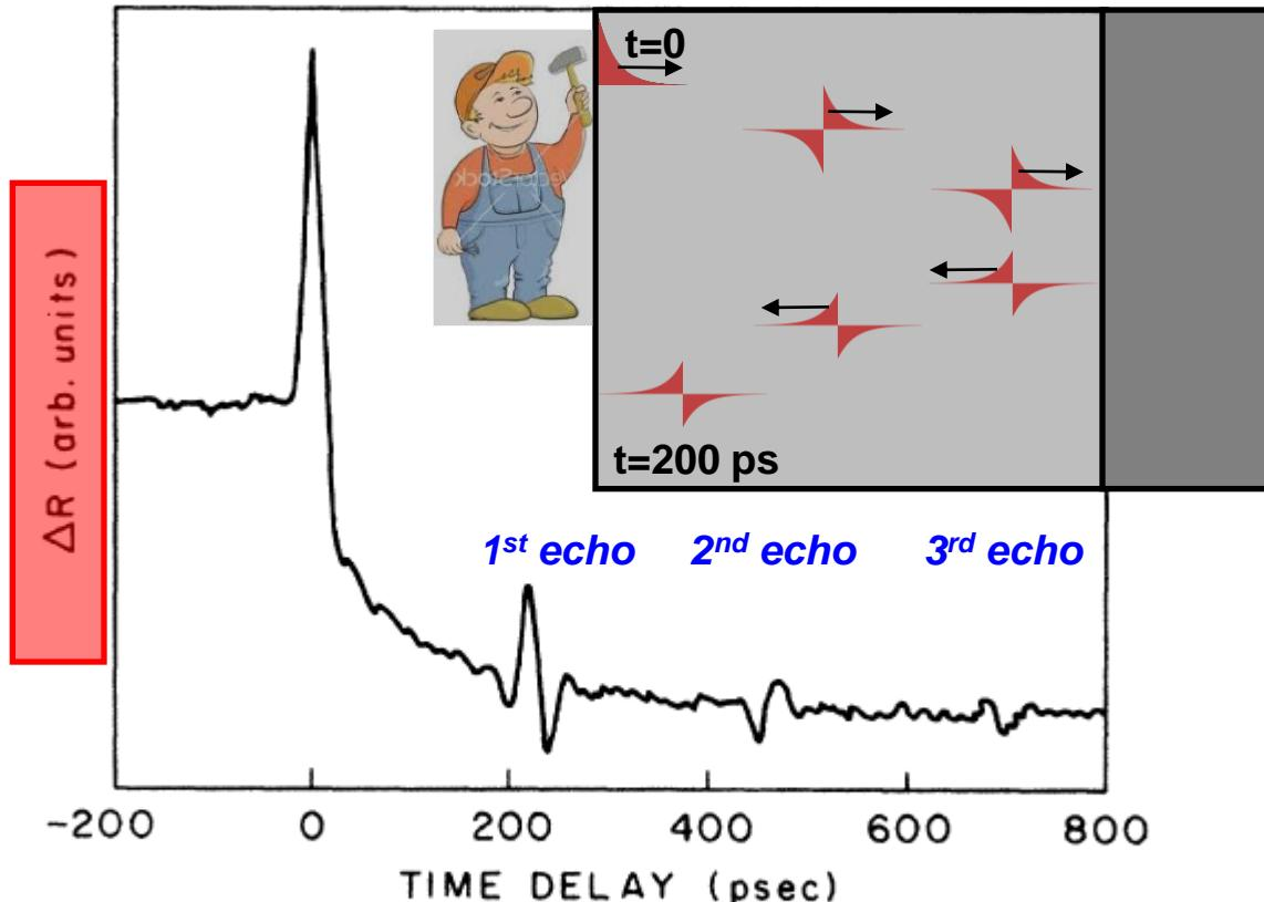
FIG. 4. Photoinduced changes in reflectivity of a 2200-Å film of  $\text{As}_2\text{Te}_3$  sputtered onto a sapphire substrate.
