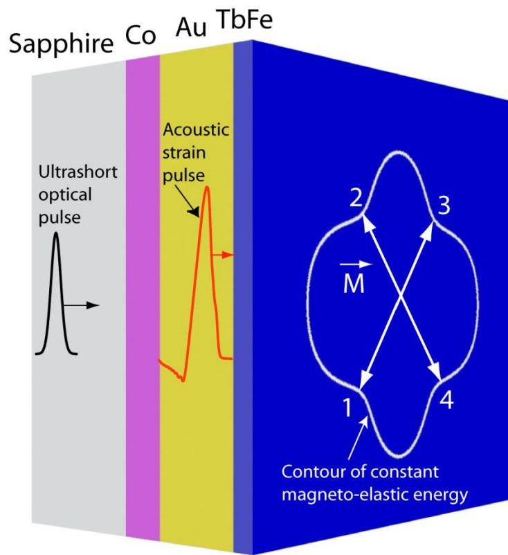
Magneto-acoustic switching for compressional ( $2 \rightarrow 4$ ,  $4 \rightarrow 2$ ) and tensile strain pulses ( $1 \rightarrow 2$ ,  $2 \rightarrow 1$ )
